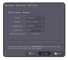
The Audio Setup tab selects the soundcard interface, sample rate, and buffer size for the session.
